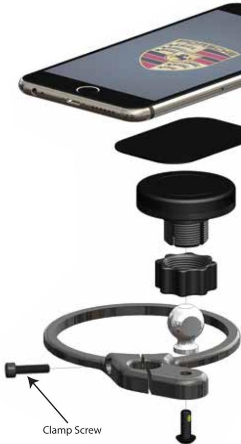
1. Install the aluminum ball onto the metal bracket as shown using the supplied screw.
