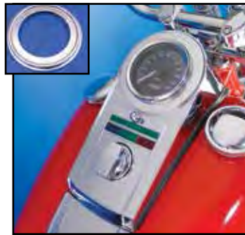
Speedometer Adapter Ring adapts to late model speedometer into FLH style steel dash cover. FLH Dash is shown with adapter ring installed VT No. 39-0130, adapter ring must be affixed with an industrial adhesive for a leak proof seal. VT No's 39-0124 and 39-0192 include chrome ring and bracket to mount electronic speedometer in FLH style dashes.
