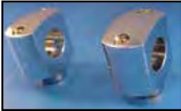
Shorty Riser Set features 1" rise with 1/2" — 13 threads for handlebars. VT No. Finish 25-2184 Chrome 25-2221 Black
