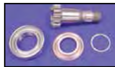
WR 3rd Gear includes bushing and washer. VT No. 49-0598
